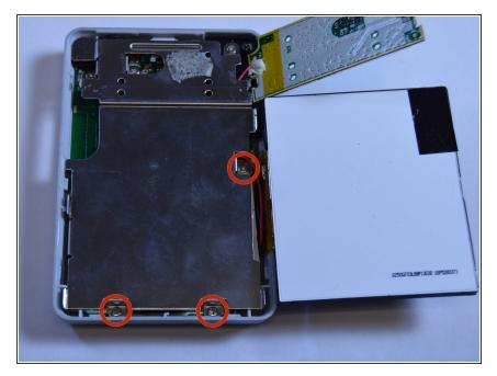
Use a Phillips Head screwdriver to unscrew the three 3/16 inch screws that were underneath the LCD screen.
