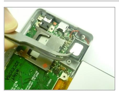
With the speaker exposed, use a pair of tweezers to lift the speaker out of the slot. To reassemble your device, follow these instructions in reverse order.
