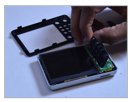
The black rubber button pad can be removed by simply picking it up.
