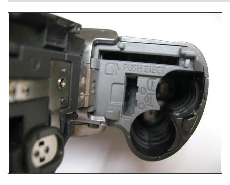
To replace the memory card, make sure it is oriented with the label facing towards the front of the
