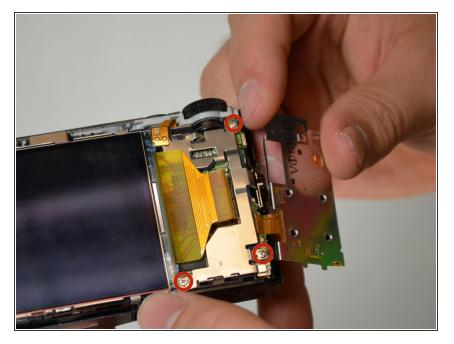
Remove the three 4 mm screws with a #00 Phillips screwdriver.
