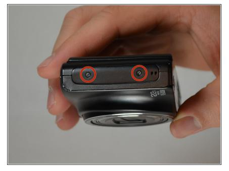
With the screen facing you, locate the two 3.5 mm screws on the left face of the camera. Remove them using a #00 Phillips screwdriver.
