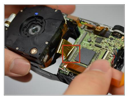
• Detach the ribbon cable connecting the lens unit and circuit board.
