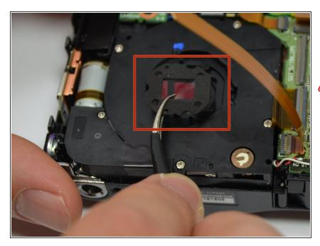
Using tweezers, remove the lens cover from the lens.
