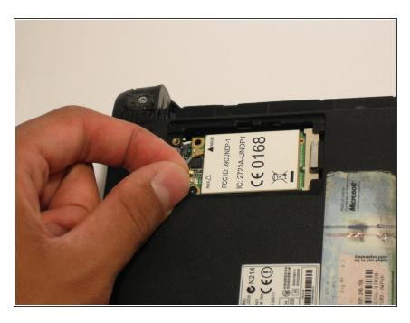
Disconnect the two antenna cables from the left side of the wireless card.
