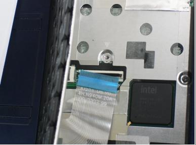
Disconnect the ribbon by lifting the black plastic hinge and removing the clear blue cable.
