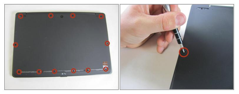
Starting with the laptop top-down, locate and remove the twelve 1mm Phillips #0 screws securing the back cover to the main body of the computer.
