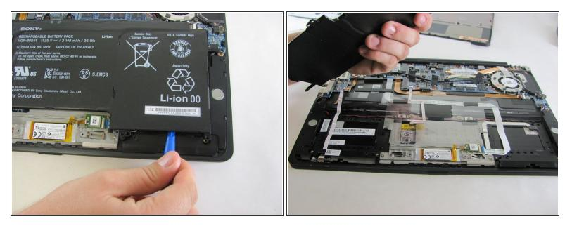
Remove the battery with the Plastic Opening Tool by placing the tool between the battery and the computer and cautiously prying it out.
