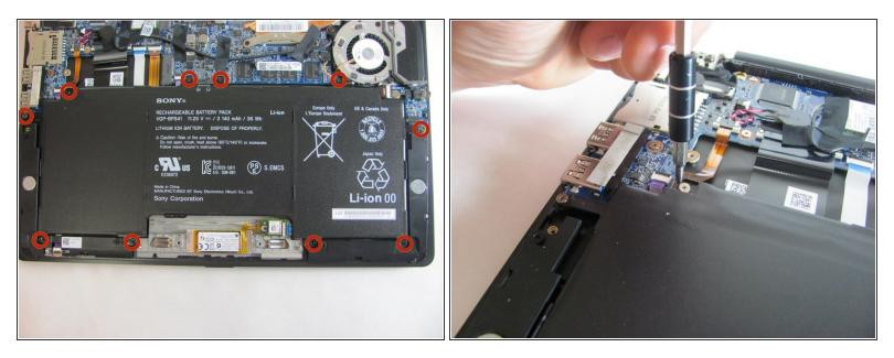
• Locate and remove the ten 1mm Phillips #0 screws that are securing the battery in place.
