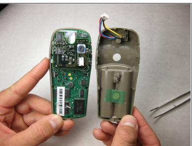
With tweezers (or your fingernails), carefully disconnect the wires between the PC input and the motherboard.
