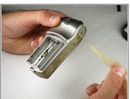
With the pick side of a spudger (or tweezers), peel the sticky tape from the device.
