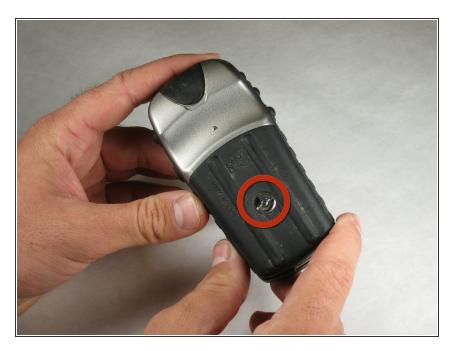
Flip the device to the backside, and locate the metal tab at the center of the back cover.
