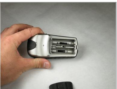
Lift the battery plate off to either insert or remove 2 AA batteries.
