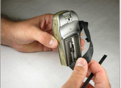
With the wedge side of a spudger (or a small, flat head screwdriver), remove the black rubber case support from the device body.
