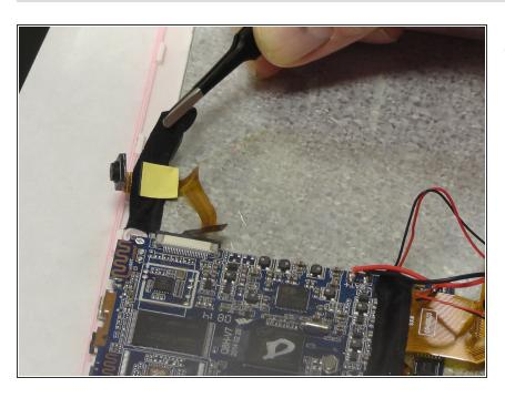
Use tweezers to remove the black tape holding the camera down.
