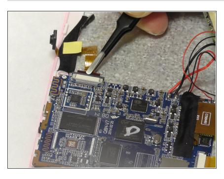
Use small needle nose pliers to carefully remove the yellow ribbon attached to the motherboard.
