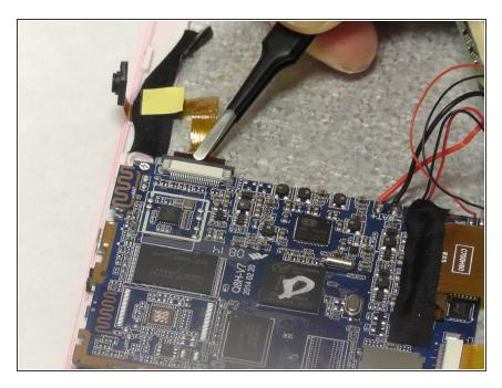
Slot the new dual camera ribbon into the motherboard.
