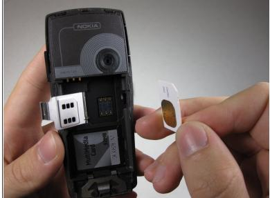
• The SIM card, now released, can easily be lifted out of the phone.
