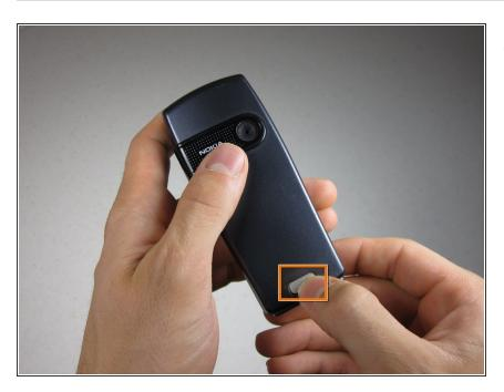
Press down the button on the back panel.
