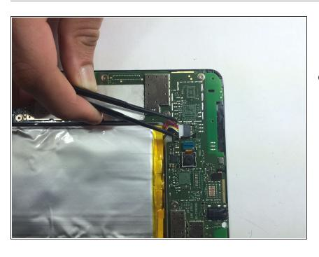
Gently disconnect the battery from the motherboard using your fingers or a pair of tweezers.
