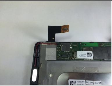
Use a spudger to remove the ribbon cable that is around the speaker wire.
