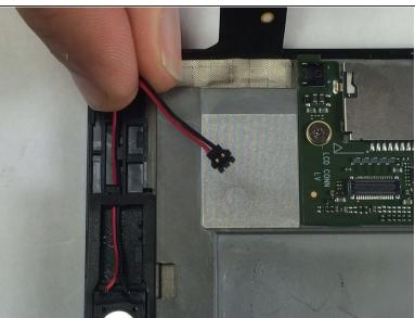
Disconnect the speaker wire from the motherboard by prying the connector upwards with the spudger.
