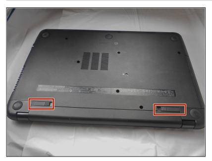
There are two battery release switches circled.
