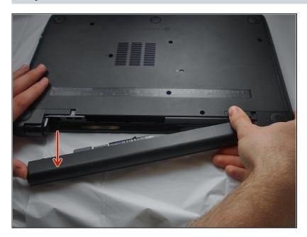
after sliding the release switches, pull battery towards yourself to remove battery.
