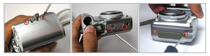
Remove the six 4 mm screws from the sides and bottom of the camera with a Phillips #00 screwdriver.
