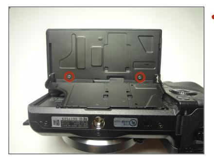
• Remove the two 1.0 mm Phillips #00 screws from back of the LCD screen.
