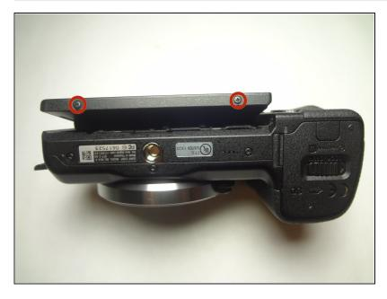
Remove the two 1.5 mm Phillips #00 screws from the bottom of the screen mount assembly.
