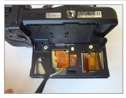
• Lift and slide out the upper black plastic separator using tweezers.
