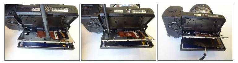
• Using the flat end of the spudger, push on the black nylon sheet glued to the metallic frame to peel it of.
