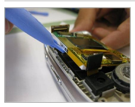
Use a spudger to lift away the LCD screen.
