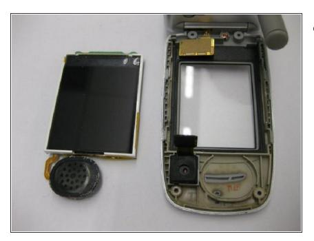
LCD screen successfully removed!
