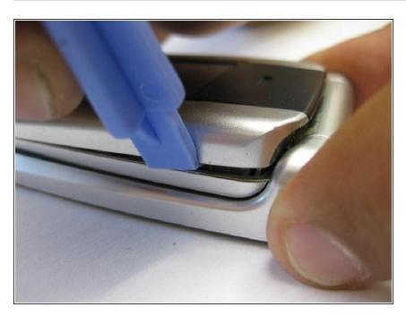
Use a spudger to pry the front cover off of the phone, gradually working your way around the front face.
