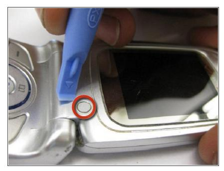
With phone in the flipped-open position, use a spudger to remove the four (4) rubber pads (one shown in red circle) located near the corners of the face with the LCD screen.
