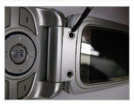
Use a small Phillips head screwdriver to remove the four (4) screws exposed by removed rubber pads.
