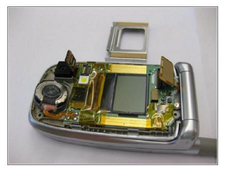
This is what the rear of the LCD screen should look like before proceeding. Note all necessary connections are undone.
