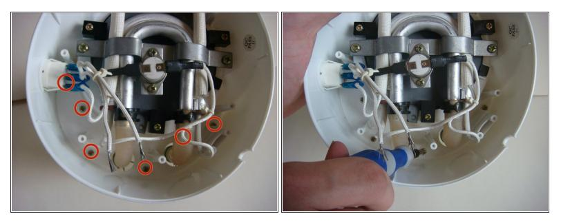
• Using a Phillips #1 screwdriver, remove the six 12mm screws.
