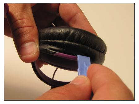
Then take one of the plastic opening tools, and apply fabric back into plastic slot from which it was removed as shown. Wedge fabric back into plastic along the entire circumference of plastic ear-cup.
