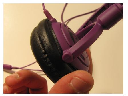
Now that the padding has been completely removed, take the new ear pad, and wrap the fabric completely around the plastic earcup as shown.
