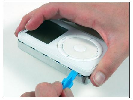
• Continue to run the opening tool along the side of the case until all five tabs have been released.
