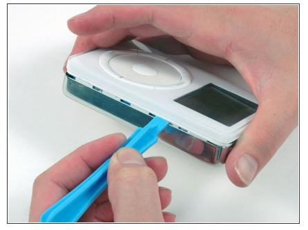
• Free the five tabs holding the iPod together on the other side. You may be able to free the tabs by gently wiggling the front panel of the iPod.
