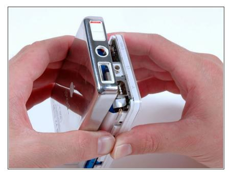
• Lift the rear panel away from the iPod, making sure it doesn't catch on the headphone jack.
