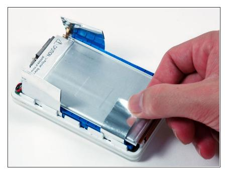
• Peel up the metallic tape attached to the top of the battery.
