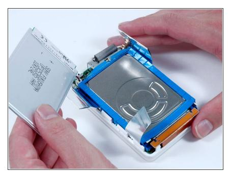
• Lift the battery up from the hard drive and lay it next the the iPod (it is still connected to the logic board).
