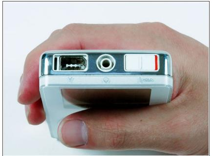
*i* Before opening your iPod, ensure that the hold switch is in the locked position.
