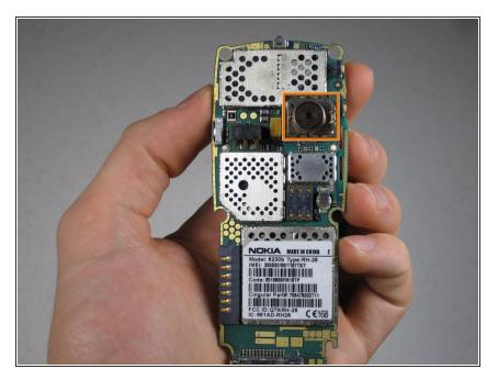
Locate the camera on the circuit board.
