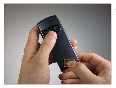
Press down the button on the back panel.
