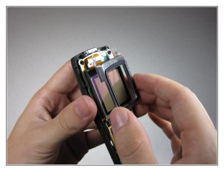
• Remove the LCD screen frame.
