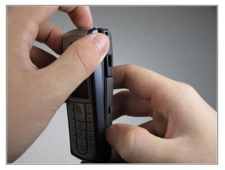
Slide your thumbnail down the case seam to separate the rest of the case.
