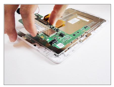
Carefully lift the motherboard directly up.
