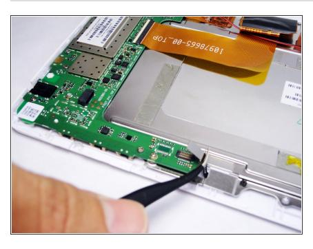
Gently pry the front facing camera plug up and off of the motherboard.
