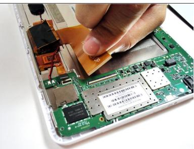
Remove the larger ribbon cable by gently flipping the beige latch and pulling it out with tweezers.
