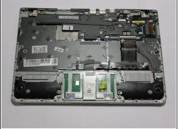
Unscrew the four 3.7 mm screws holding down the speakers using a Phillips #00 screwdriver.
