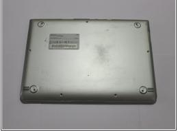
Remove the nine 4.7 mm screws on the bottom cover using a Phillips #00 screwdriver.
