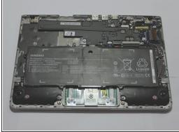
Pry off the bottom cover using a plastic opening tool.
