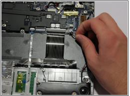
Disconnect the cable connecting the speakers to the motherboard by pulling on it away from the motherboard.
