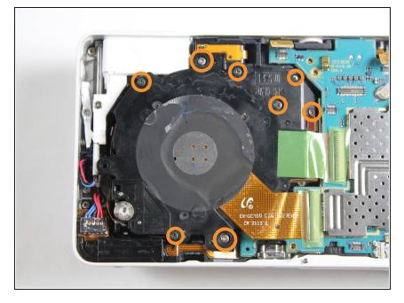
Unscrew the lens' screws. There are 1 black 4/32" screw, 3 3/16" black screws, and 2 white 5/32" screws.
