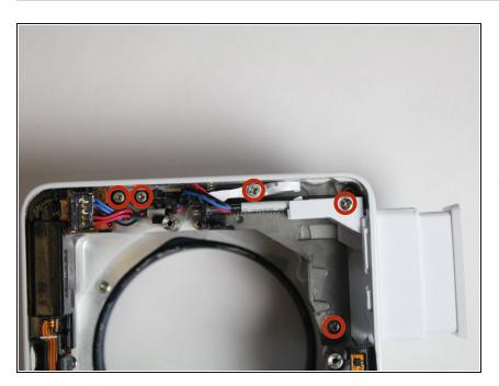
Remove all the screws circled. There is 1 1/8" screw by the flash, 1 9/32" screw that holds the flash button, 2 5/32" screw that is on the
