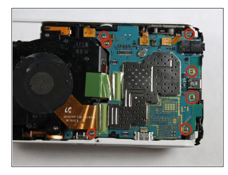
Unscrew the motherboard's screws. There are 4 3/32" screws and 3 5/32" screws.
