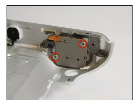
• Unscrew the 2 5/32" screws on the grey plate.
