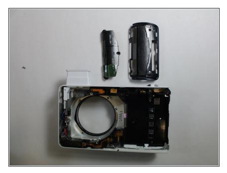
• The black plates on the other side can be removed after these screws.
