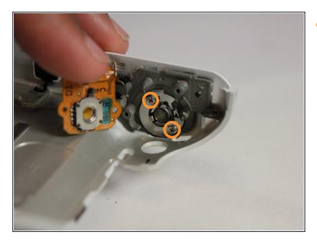
Pull the plate aside and unscrew 2 1/8" screws on the button.
