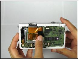
• Remove the black rubber tape with the plastic opening tool and slowly peel it off.
