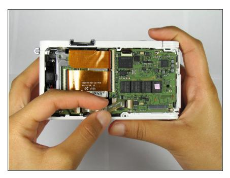
Disconnect the bottom ribbon by grasping the ribbon and wiggling it out gently from the connection.
