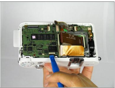
Carefully place the motherboard back down to remove the last ribbon. Lift the black latch up from the ZIF connector of the last ribbon with the plastic opening tool.
