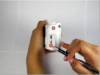
Unscrew the three 4.5mm #000 Philips screws on the sides of the camera using the Philips #000 screwdriver.
