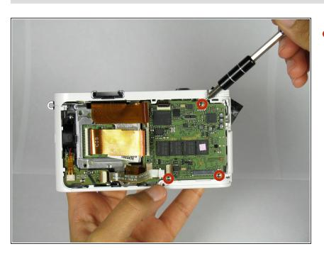
Unscrew the three 4.5mm Philips #000 screws with the Philips #000 screwdriver.
