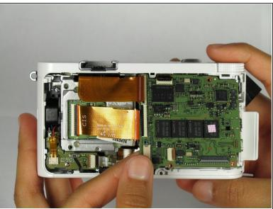
Using the plastic opening tool lift the motherboard up starting from the bottom left side.
