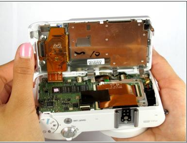
Open the two halves of the camera, taking care not to disturb the ribbon cable.
