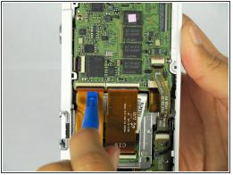
Open the ZIF connector on both of the larger ribbons by lifting the black latch with the plastic opening tool.
