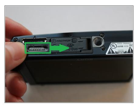
On the bottom of your camera, slide the gray lock in the direction of the pointed arrow. This will open the battery hatch.
