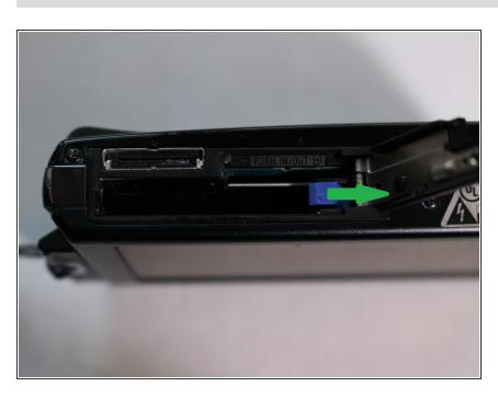
On the inside of the battery compartment, there is a small blue lever. Push this lever back to release the battery.
