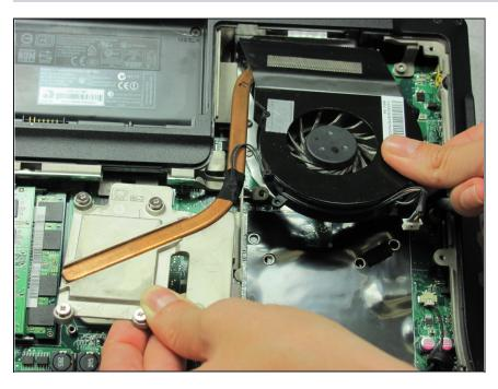
• Pull the fan and heat sink toward you at a 20 degree angle upward.
