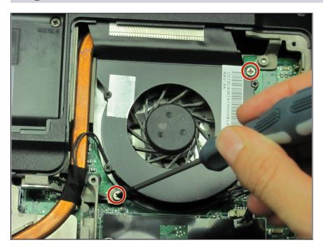
Remove the two screws located on opposite sides of the fan with a Phillips #00 screw driver.
