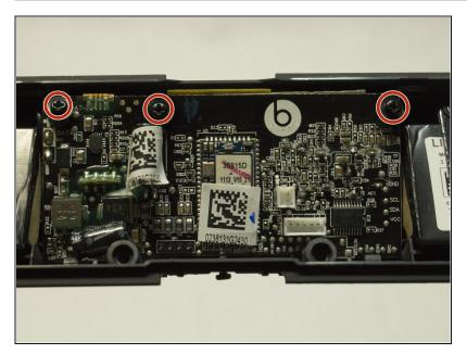
Remove the three 9 mm screws from motherboard and rubber stopper using a Phillips #0 screwdriver.
