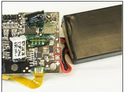
• Using a wire stripper, cut the red and black wires attached to the motherboard.
