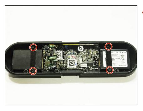
Using a <u>Phillips #0 Screwdriver</u>, unscrew the four screws holding the bands that go over the battery.
