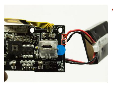
Cut off the battery wires
