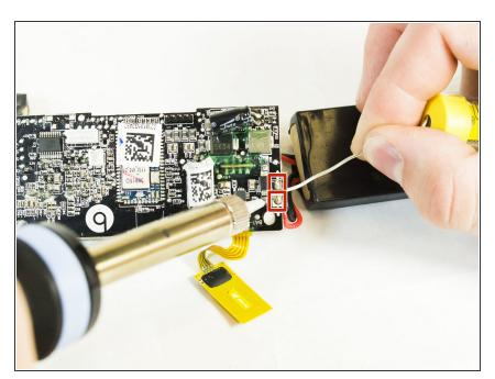
Using a soldering iron attach the new battery to the motherboard with the red wire connecting to the 0.2 volts (+) and black wire connecting to the ground (-). See the <u>soldering</u> <u>guide</u> for more information on how to perform this step.
