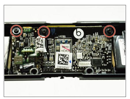
Using the same <u>screwdriver</u>, remove the motherboard screws along with the rubber stoppers.
