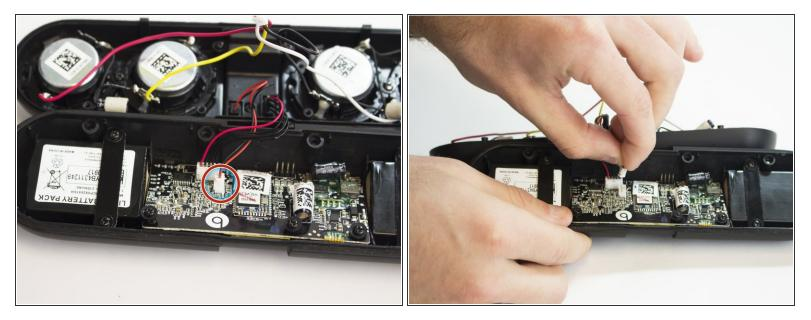
Carefully remove the black and red NFC sensor wires.
