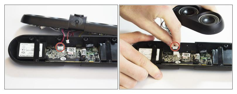
• Carefully remove the control cables (4 black, 1 red).
