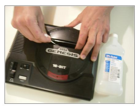
Rub a Q-tip dipped in rubbing alcohol along the pins of the cartridge slot to remove any remaining debris.
