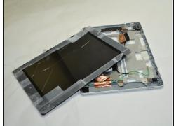
• While holding the side of the screen, press the metal plates behind the device to pop the screen out.
