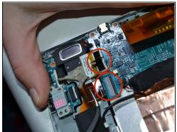
• Continue to disconnect all resistors attached from the motherboard, using tweezers.
