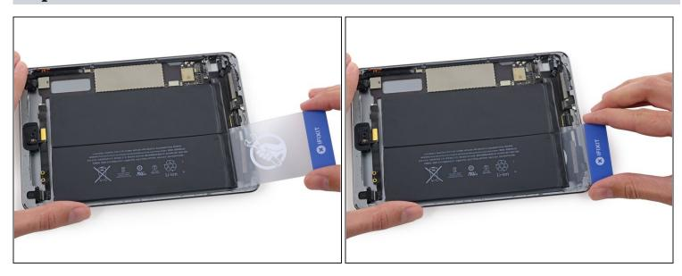
• Remove the plastic card and insert it under the battery cell nearest the edge of the case.
