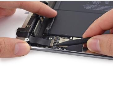
• Use the tip of a spudger to lift the LCD connector up off its socket on the logic board.
