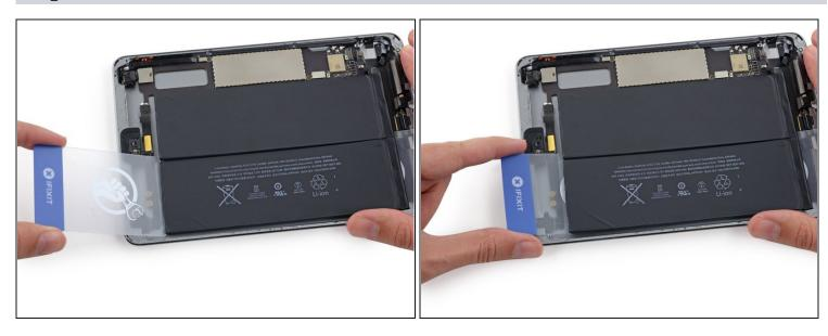
• Remove and insert the second card under the battery near the headphone jack.
