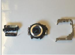
Now, the flash assembly and metal frame can be easily pulled away from the lens.
