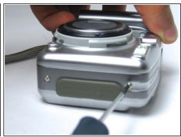
Use the Phillips #00 Precision Screwdriver to remove the six 4 mm Phillips head screws found on the sides and bottom of the camera.
