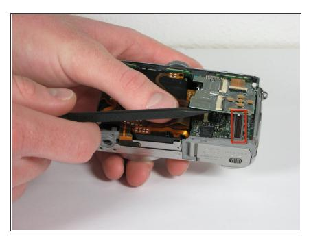
Carefully unsnap the front logic board from the rear logic board using a spudger.
