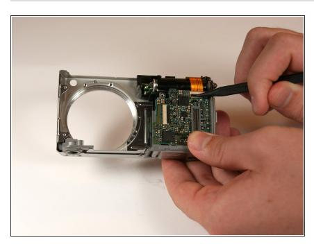
Use the spudger to unclip the top ribbon cable from the circuit board.
