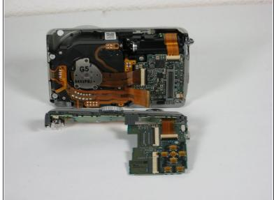
Slide the entire top part of the camera that is attached to the logic board, horizontally away from the camera.
