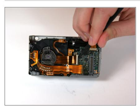
Use a spudger to detach the ribbon cable from the circuit board. Lift the black clip up to unlock it as before.
