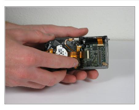
Push the lens assembly slightly toward the circuit board, and pull the left side out of the casing first. You will have to wiggle this out gently.
