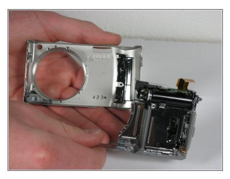
Remove the front casing from the rest of the device.
