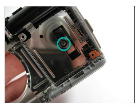
Remove the 3.5mm colorless screw that lays within the square opening of the inner casing.
