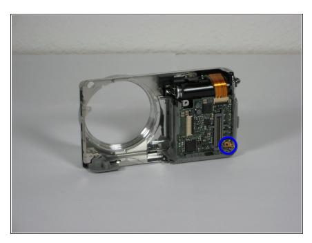
Remove the single 2mm screw in the bottom right corner of the circuit board
