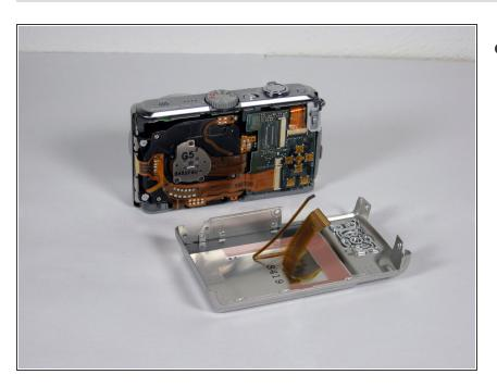
Remove the back casing from the camera.
