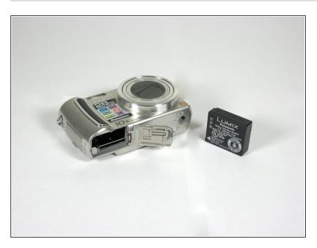
Remove the battery and memory card from the device.
