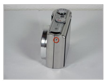
Remove the single 3.4mm screw on the left side of the camera.
