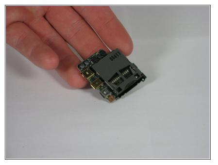
Take note of how the slots fit into the circuit board for easy replacement.
