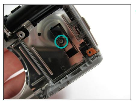
Remove the 3.5mm colorless screw that lays within the square opening of the inner casing.
