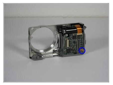
Remove the single 2mm screw in the bottom right corner of the circuit board
