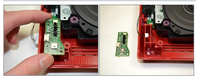
Lift the power board from the console and set it aside.
