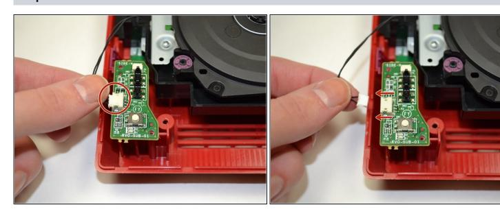
Using your fingers, gently pull the pin connector to disconnect the power board from the disc drive.
