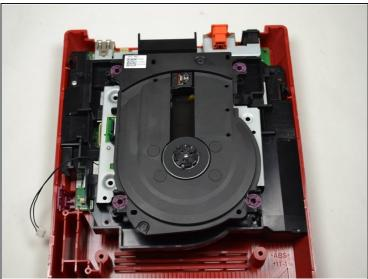
Using a Phillips #0 Screwdriver, unscrew the four 6mm screws.
