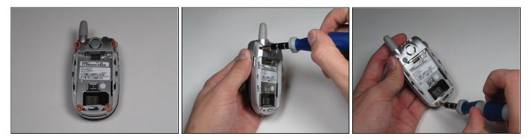
• At the corners of the phone, remove all four 6.0 mm Torx screws, using your screwdriver.
