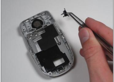
• Using metal <u>tweezers</u>, lift out the black plastic support piece from beneath the headphone jack.
