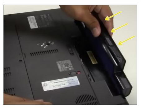
Insert the new battery into the slot. Push the Gateway MD2614U battery towards the laptop and secure it in place.
