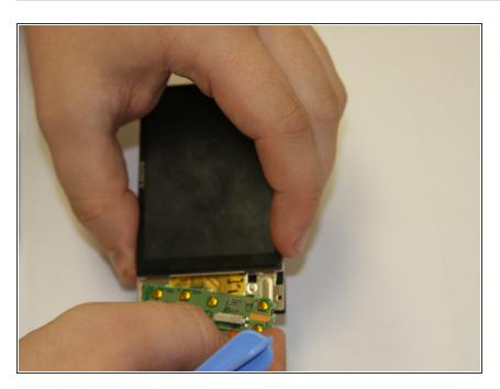
Remove the button circuit board.
