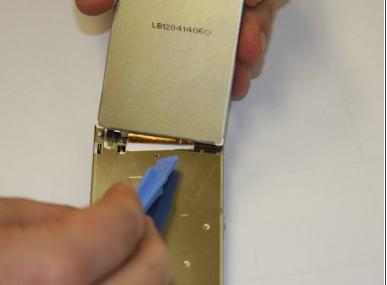
• Use spudger to pry apart the LCD screen from the support bracket.
