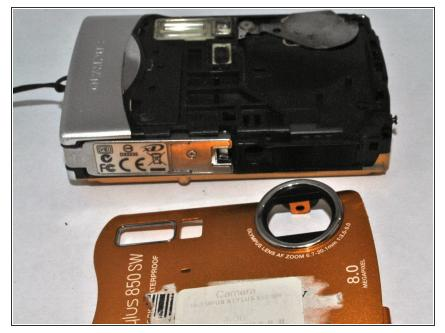
First, we need to get inside the camera. Refer to the <u>lens cleaning</u> <u>guide</u> for steps on how to remove the front panel.
