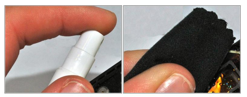
Remove the keys and clean using solution and a soft cloth. If the keys are damaged, you will need
