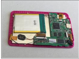
Remove the tape holding the motherboard, wires, and connecters in place.
