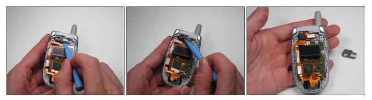
• Use a plastic opening tool to dislodge and remove the rubber camera cover.
