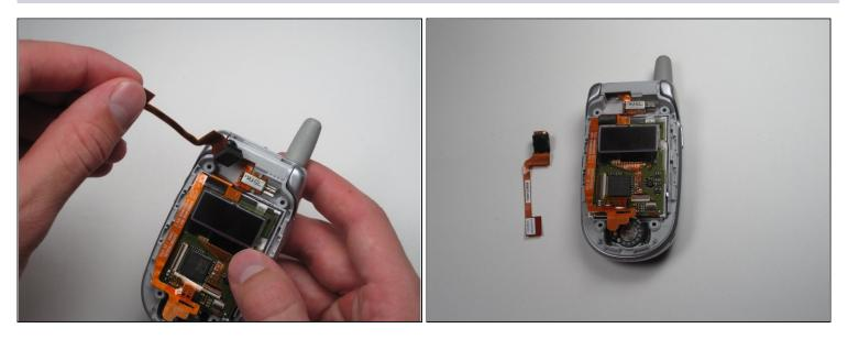
• Lift the top ribbon cable, with camera attached, up and away from the rest of the phone.
