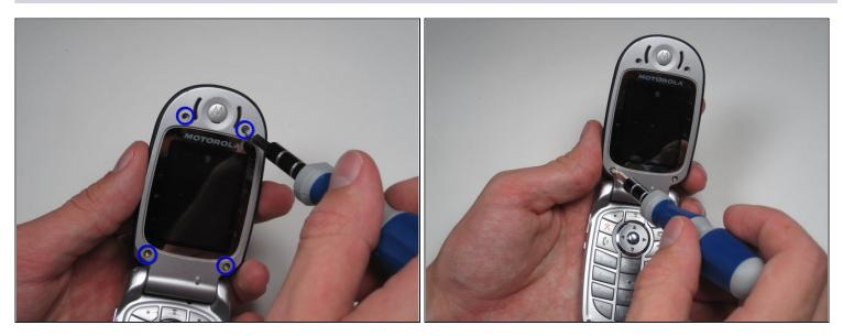
• Remove the four 3.8 mm T-6 Torx screws.
