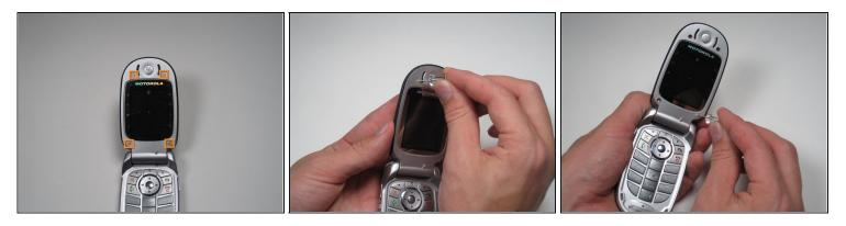
• Remove the four rubber stoppers from around the screen with a pin to reveal four screws.
