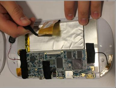
Flip up the retaining tab (the black bar on the connector), then pull LCD connector with tweezers.
