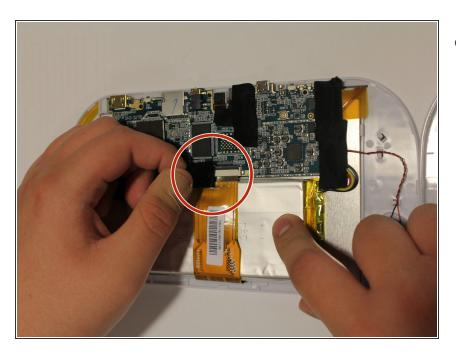
Remove tape from the LCD connector.
