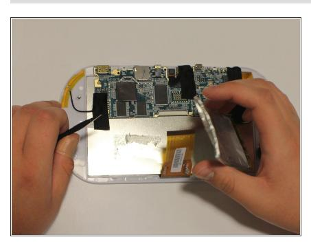
Now remove battery. The battery should still be pried from the LCD display, if not pry it again.
