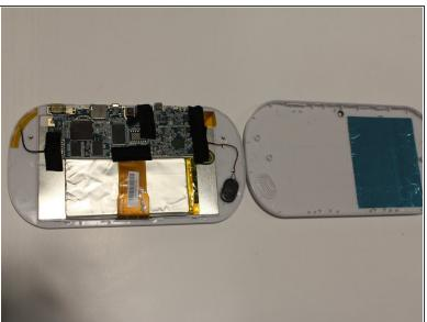
Pry open the Ematic FunTab 2 using the plastic opening tool.
