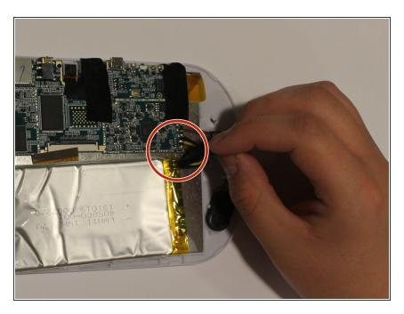
Remove tape from the yellow, red, and black wires connecting the battery to the LCD.
