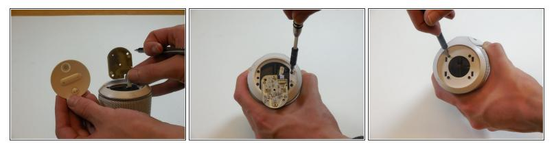
Unscrew four 3.3mm screws on each end of the JBL using a size 1 ph screw driver (8 screws total).
