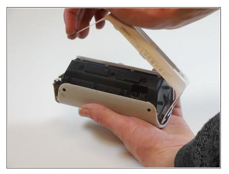
Remove last white back plate to expose the back of the speaker cover.
