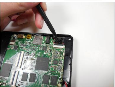
Gently pry the front-facing camera away from the back panel using a spudger.
