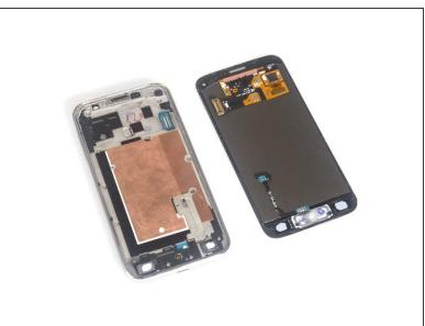
Remove the LCD screen from rear case.
