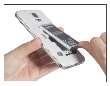
Remove battery. If you have SIM card and SD card in, remove them by the way.
