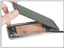
• Heat the screen, cut the sticker under it and release the screen connector. Please be careful with the screen flex when sliding to cut the sticker.
