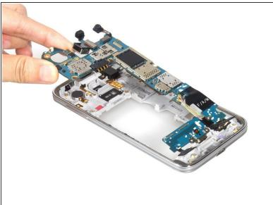
Twist off these two screws and remove the whole motherboard assembly.
