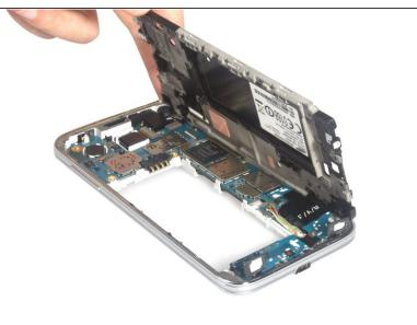
Get loosen the touch keys from adhesive, and then push the mid-plate out from the middle housing.
