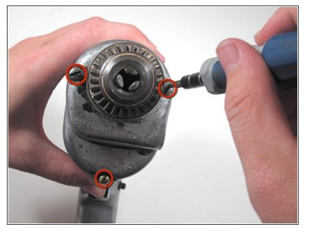
On the front of the drill, remove the three 2" flathead screws connecting the front housing to the rear housing.
