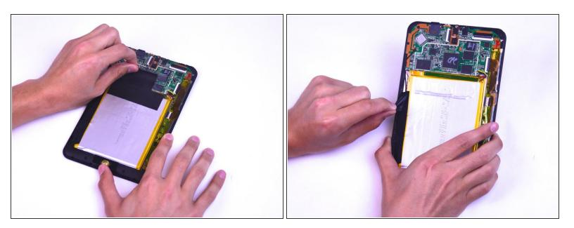
Remove the black tape that is located to the left of the device as well as the clear tape directly below the camera.
