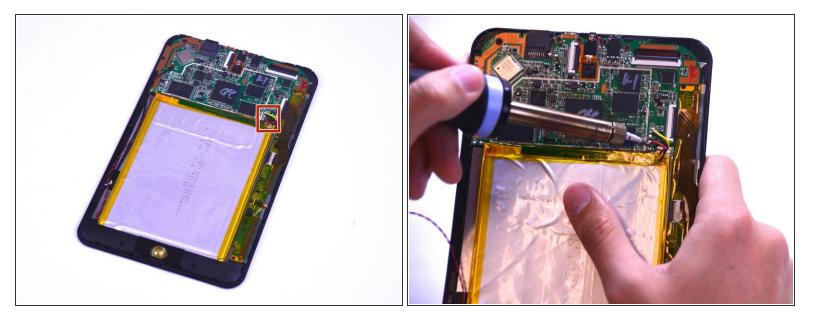
Desolder the red, black, and yellow wires to properly remove the motherboard. Take a look at this guide to learn how to solder and desolder connections.
