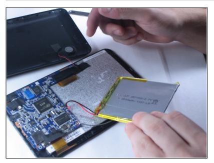
• The battery should now lift up freely from the device.
