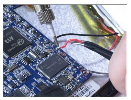
Apply heat to the solder holding each of the black and red wires to the circuit board while gently pulling with tweezers. When hot enough, the wire should pull away freely from the joint.
