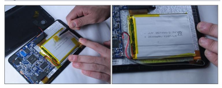
• Using <u>tweezers</u> or your fingers, begin removing the yellow tape holding the battery down to the device.
