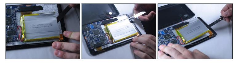
⚠ The battery is very fragile, so this process may cause some damage to the old battery during removal. Take extra care if you need the old battery to remain intact.
