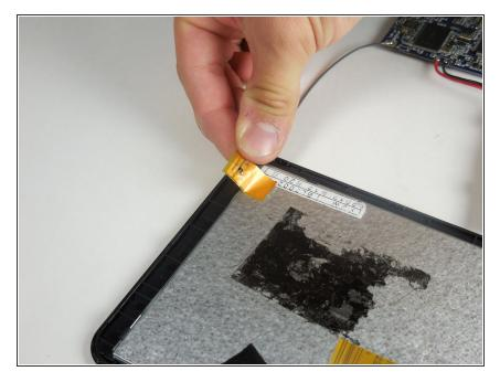
Gently peel off the orange sticker with the gray wire connected to the upper corner of the device. This is the antenna.
