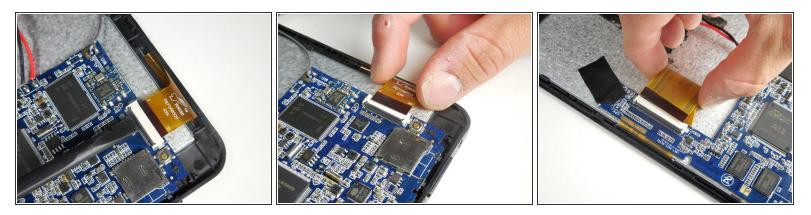
• Remove all three ZIF cables connected to the motherboard (the blue, angled piece) by lifting the gray flap with your finger or a plastic spudger and gently removing the cable.
