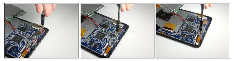
• Remove the three 2cm screws at the bottom using the Phillips PH00 screwdriver head.
