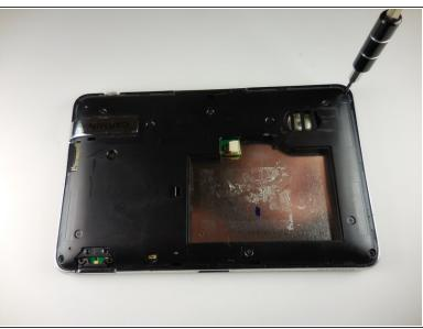
Using the T5 bit, unscrew the four 5.7mm screws in the four corners on the back of the device.
