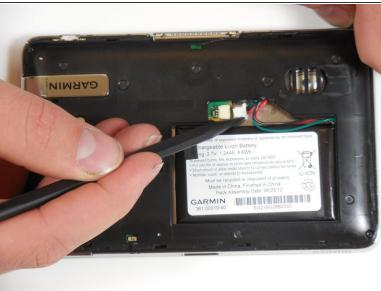
Using the plastic spudger, carefully remove the white tab connected to the battery from the device by pulling the tab in the opposite direction from which it is connected.
