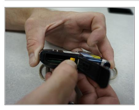
Pull orange tab to the side to release the battery.
