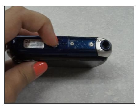
Pull down gray tab until it unlocks battery compartment.
