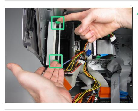
Push the two green tabs toward each other to release the optical drive and lift it out.
